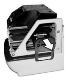
Turn the knob of the new cartridge in direction of the arrow (clockwise) to tighten the ribbon.
