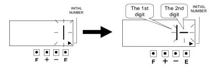
**3.** Set the correct numbers in the same manner as step 2, and then press the [E] button. When the 3rd "Number Digit" has been set at "0", then press the [E] button.
