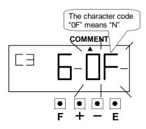
After you finished setting the customized comments, press the [E] button again, the LCD screen will return to normal mode.
