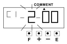
Press the [E] button, then the flashing changes from "Character Position" to "Character Code".  The 2nd character is "F", press the [+] or [-] button to set at "07", and press [E] button.
