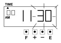
At the same time, the "Second" start to run from "00" and the LCD screen only display "▲" under the "TIME" mark.
