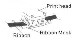
Notice: install the ribbon cartridge so that the ribbon is between the print head and ribbon mask. Printing will not come out properly if the ribbon is placed behind the ribbon mask.
